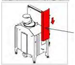
5. Attach the counterweight cover and screw in the screw(s).
