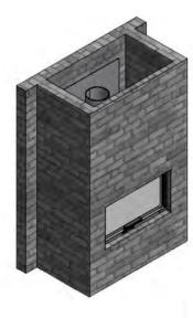
Recommended convection area is min. 600 cm² (may be distributed). Upper edge of convection outlet must be min. 200 mm from combustible material.
