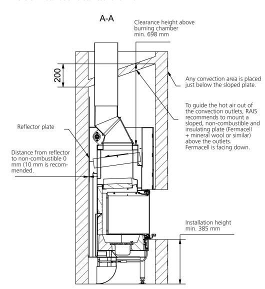
Construction of sloped plate.
