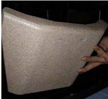
The smoke chicane rests on 2 channels. push it forwards, tilt, lower and remove.
