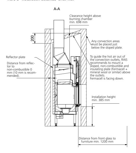
Construction of sloped plate.
