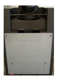
Dismount the reflector plate and turn it upside down. Mount the plate by reusing the screws at the bottom.
