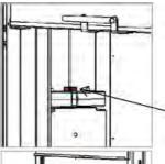
4. Tighten the retaining ring (Allen key 2.5mm).
