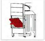
1. Remove the Side Skamol sheet.
