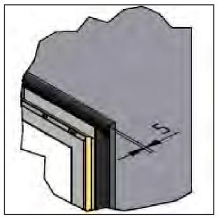
Due to the stoves structure there will be air gaps of 26,5 mm to the sides and the bottom, which can be closed e.g. with non-combustible panels.
