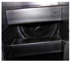
When remounting the chicane, secure the plate under locking plate.
