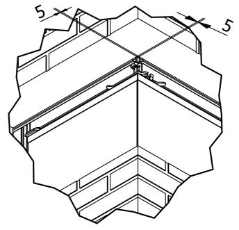
Due to the stoves structure there will be air gaps of 34 mm to the sides and the bottom, which can be closed e.g. with non-combustible panels.
