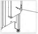
1. Remove the transport lock and the screws on the counterweight cover
