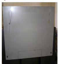
Bend the cut-outs and mount the plate to the top of the stove.
