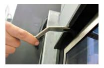
The side glass is released by wrenching the bracket below and above the side glass.
