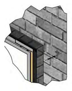
Due to the stoves structure there will be air gaps of 26,5 mm to the sides and the bottom, which can be closed e.g. with non-combustible panels.
